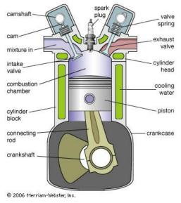
exhaust gas escape while the engine is in operation. At the top of a cylinder sit two valves - one for letting fuel in (**intake**), the other for letting exhaust gas out (**exhaust**) - and a spark plug, which is a device for introducing a spark into the cylinder to explode fuel.
