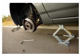
**First**, find a safe place to do the work. You might need to move the car, if you are on a dangerous section of road. A safe place should be safe for you to work, and have a flat, strong, level (not on a hill!) surface on which to place the jack. You are going to be lifting the car with the jack - it **must** be stable **at all times**!
