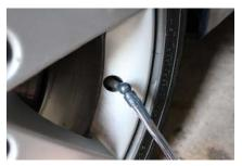
You can check to see if a tyre matches the correct pressure by using a **pressure gauge**. These are simple devices that you connect to the valve of the tyre. Shown here is an analogue pen gauge, but you can get digital dial versions too. If the tyre doesn't have enough air, you can add more by using a pump.
